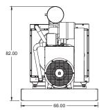
Drawings based on standard open power 480 volt standby generator. Lengths may vary with other voltages. Subject to change without notice. Sound data as measured at 23 feet (7 meters) in accordance with ISO 8528-10 at standby rating.
