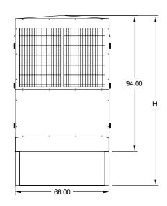
All enclosure models are 200 MPH wind rating certified in accordance with IBC2018 and ASCE/SEI 7-16 standards.
